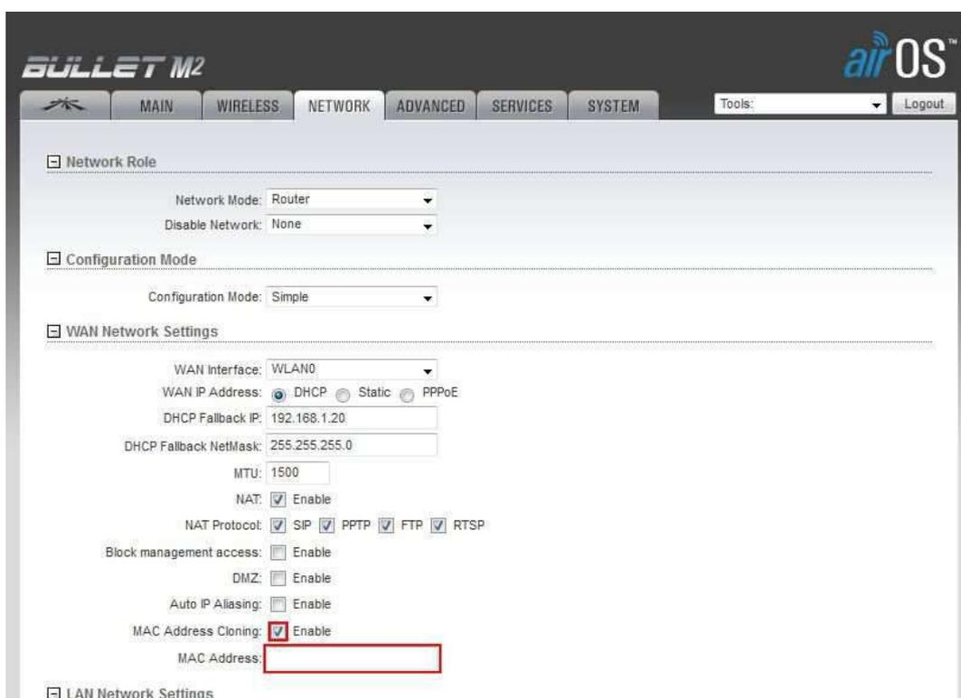
The screenshot shows the web interface for a Bullet M2 device. The 'NETWORK' tab is selected. Under 'WAN Network Settings', the 'MAC Address Cloning' checkbox is checked, and the 'MAC Address' field is highlighted with a red box. Other settings include 'WAN Interface' set to 'WLAN0', 'WAN IP Address' set to 'DHCP', and 'NAT' enabled.
